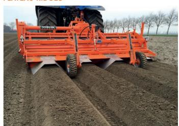
Stainless steel insert plates on the press units for making plateau-ridges, in which you can plant directly.
