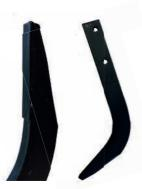
Widia hook, suitable for all types of soil that is free of stone – three times as hard wearing than a double welded tine, and its correct angle of contact at 14° makes sure the ground is broken open instead of compacted.
