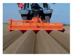
The Struik ridging system provides voluminous ridges with a capacity of about 620 cm3.
