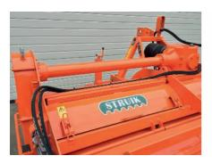
The RF hook-tine rotary cultivator is designed for high power tractors. The drive line is a combination of a gearbox and a chain drive.
