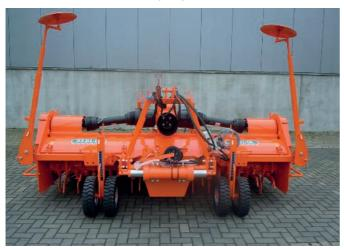
With modifications to the standard frame, the RF is available with a double-sided drive in combination with a maintenance-free centre bearing and a Cat. 3 tensioner.
