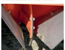
Subsoilers in the hood provide better water drainage between the ridges. The additional loose soil created prevents drying out in the worked channel.
