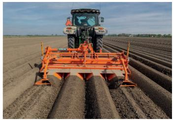
Handle riding tracks easily and quickly with the hydraulic or manual track scrapers.
