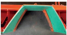
The ridging hood can be equipped with stainless steel press units that allows you to make ridges at a higher speed, and they will keep their shape. With the steel press units coated in Multilene, wear and mud build-up are things of the past. Capacity increases up to 25% are achievable with both systems.
