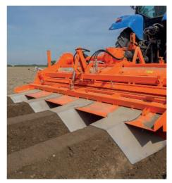
The ridging unit can be equipped with an automatic regulator that maintains constant pressure on the ridging hood, and that produces a lasting ridge with a rigid shape.
