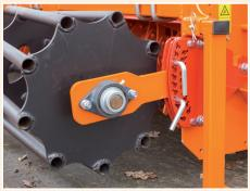
Pin-hole adjustment crumbler roll
